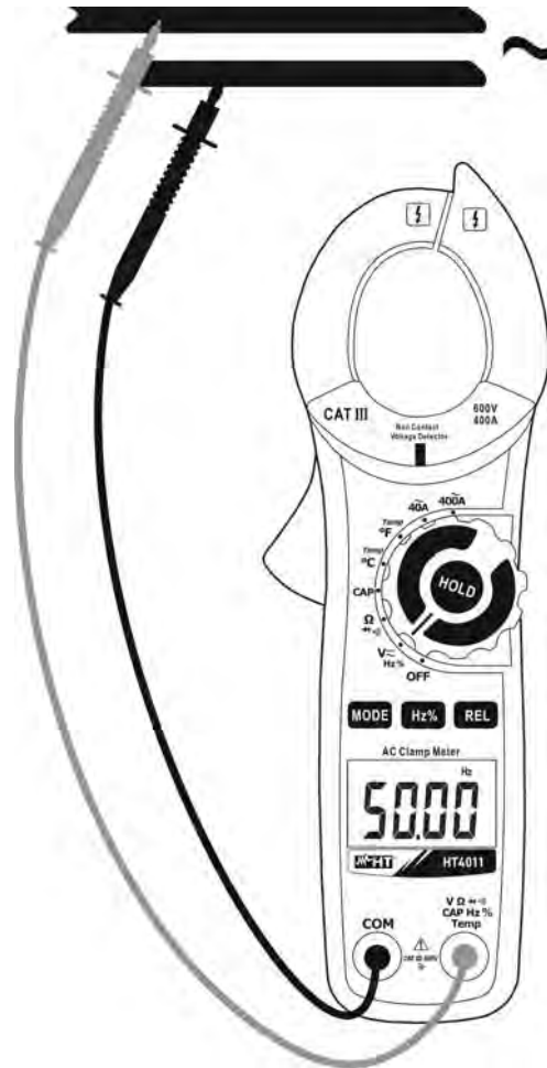
Fig. 4: Use of the clamp for frequency measurement and duty cycle
