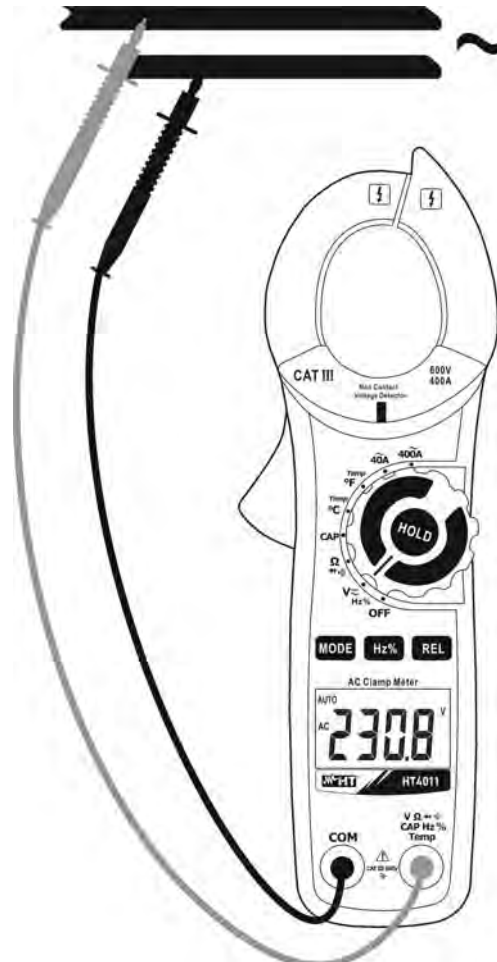
Fig. 3: Use of the clamp for AC voltage measurement
