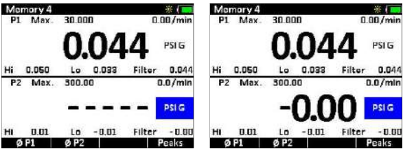
Zeroing the P2 sensor.
