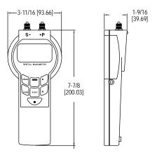
The Series HM35 Precision Digital Pressure Manometer is designed to reliably measure and log absolute pressure, differential pressure, or gage pressure with up to 0.05% accuracy. The data logging function can store up to 10,742 readings and transmit the readings to a PC through an IR serial port. The large display can graphically display trends in the data as well as peaks and valleys.
