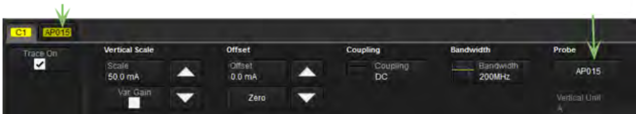
Channel dialog with tab for connected probe.
