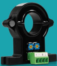
The HAK Series Hall effect DC current sensors provide precision measurements of DC current up to 1000A with a standard 4-20mA or 0-5V output signal for broad compatibility. Featuring a hinged splitcore design for fast, easy installation into existing systems, the HAK provides accurate 0.5% measurements for any DC project and is available as either a unidirectional or bi-directional device.
