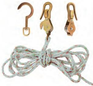
All Klein block and tackle use high-quality, 3/8" (10 mm) diameter rope. Light, galvanized-steel shell blocks are fitted with snubbing hooks to hold the load. This package features two blocks with a swivel anchor hook with a maximum safe load is 750 lbs. (340 kg).
