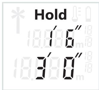
Press the “HOLD” button **1** once more to stop the measuring procedure again. The laser beam is switched off and the **HOLD** indication appears on the display. The previous measuring value is displayed in the top line. The current measuring value is displayed in the bottom line, but is no longer continuously updated.
