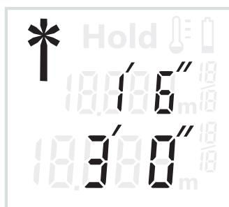
Press the “HOLD” button **1** once more to switch the laser on again. The laser indicator
