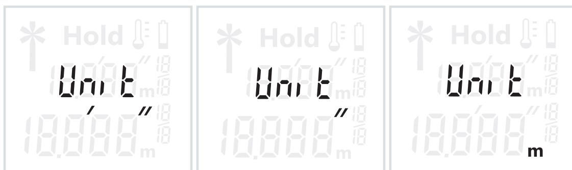
Switch off the measuring tool. Press the measuring button **1** and hold it down. The display will alternately show three units of measure. When the desired setting is displayed, release the measuring button **1**. The setting is saved.
