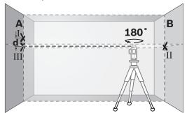
Without changing the height, turn around the tool by 180°. Direct it against the wall A in such a manner that the vertical laser line runs through the already marked point I.
