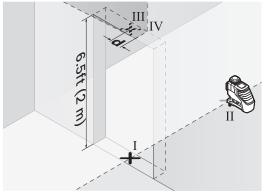
Rotate the tool by 180° and position it on the other side of the door opening directly behind point II. Allow the tool to level in and align the vertical laser line in such a manner that its center runs exactly through points I and II.
