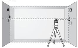
Align the height of the tool (using a tripod or by underlaying, if required) in such a manner that the cross point of the laser lines is projected against the previously marked point II on the wall B.
