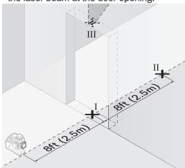
Mark the center of the vertical laser line at the floor of the door opening (point I), at a distance of 8ft beyond the other side of the door opening (point II) and at the upper edge of the door opening (point III).
