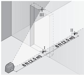
Mark the center of the vertical laser line on the floor of the door opening (point I), 16 ft (5 m) away on the other side of the door opening (point II) and on the upper edge of the door opening (point III).
