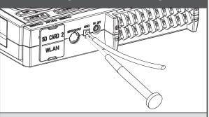
Use a flathead screwdriver to push the button above the GND terminal while connecting the grounding cable to the GL260.
