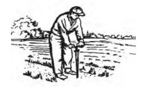
Using a soil auger, soil sampler, or posthole digger, you can insert Delmhorst Gypsum Blocks at any depth to best suit the root structure of each crop, since moisture is checked in areas of active root growth.
