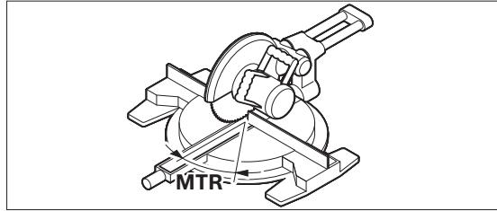
Press button **14**. The calculated horizontal miter angle “**MTR**”, which has to be set on the chop and miter saw, and the “**MTR**” indicator will be shown on the display.
