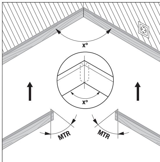
The miter angle “**MTR**”, by which the two workpieces are to be shortened, is calculated. For these miter cuts, the saw blade is vertical to the workpiece (the bevel angle is 0°).
