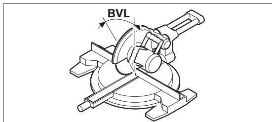
Press button **15** again. “**BVL**” and the calculated bevel angle for the chop and miter saw is indicated on the display. If required, the miter and bevel angle can be recalled again, but only as long as button **12** for changing the operating mode has not been pressed. Press button **15** to recall the angles. “**MTR**” and the calculated miter angle are indicated in the display; after pressing the button **15** once more, “**BVL**” and the bevel angle will be indicated.
