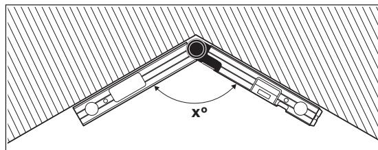
When workpieces are to be fitted into a corner (e.g. for floor trimmings), measure the corner angle  $x^\circ$  by applying the fold-out leg and the base leg. For given angles (e.g. picture frames), open the fold-out leg and the base leg until the desired angle is indicated in the display.
