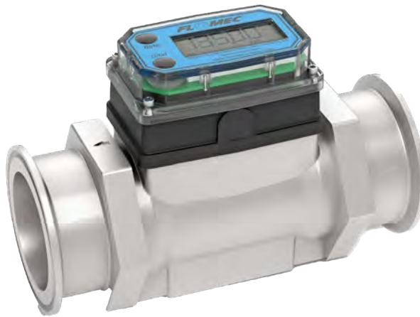
The FLOMEC® G2 Brew Meter features a high-temperature riser and Tri-clamp fittings. It is suitable for use with strike water, hot water flow, and brewing liquids.
