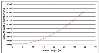
Max. camber = 0.020 in. x (length in feet)<sup>2</sup> or 0.005 in., whichever is greater.
