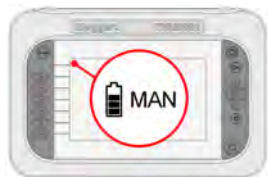
Current operational state. Currently in Manual operation
