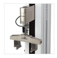
Series FS06 sensors are suitable for bulkier grips and fixtures, such as the G1095 bend fixture and eye end adapter shown here.
