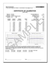
Included certificate of calibration contains 10 data points in each measuring direction.
