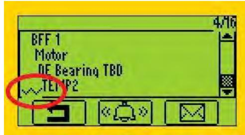
Checkmark indication applies to all measurement settings/sensors.
