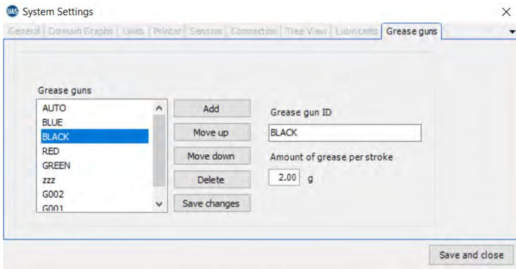
When done, left click on ADD. You can sort your list by selecting any grease gun and moving it UP or DOWN with the move up/move down buttons. You can also Edit grease gun IDs or delete them altogether. Left click Save to save your changes or the "X" in the top right to exit without saving.
