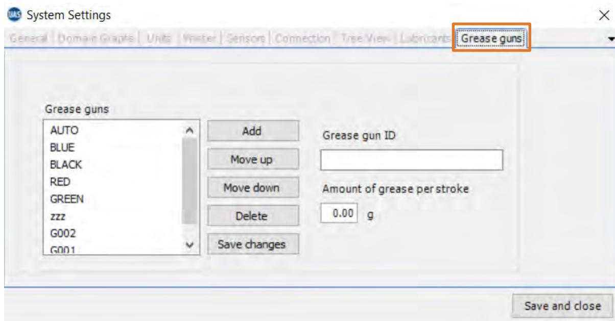
UAS3 and LUBExpert want to ensure you always use the right grease and the right amount. To accomplish this, you need a tool to manage your grease guns. To manage multiple grease guns in
