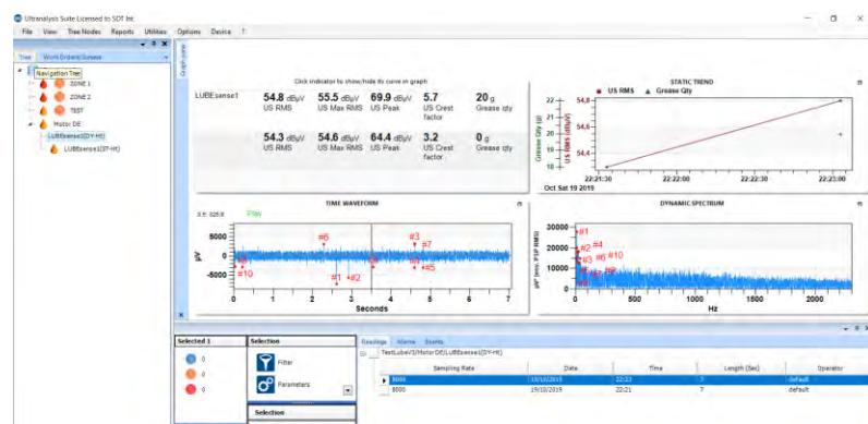
Two Dynamic measurements are collected during initial and final reading of your lubrication process, thus describing condition of your bearing before and after the grease replenishment process. This is great data the lubrication technician provides directly to the condition monitoring team.
