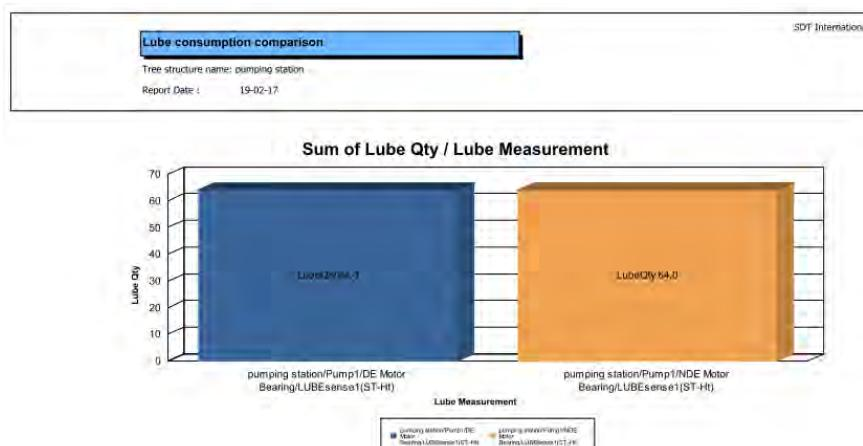
The generated report details the lubricant consumption per lubrication point for the chosen period.
