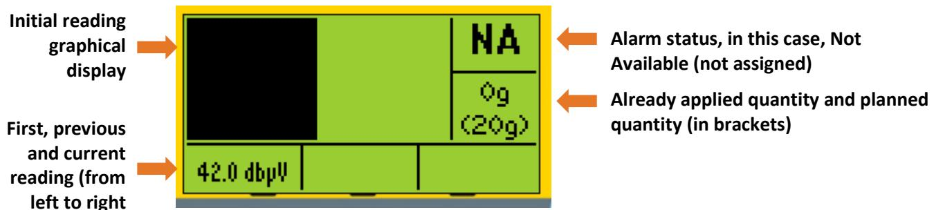
(In cases when alarm is assigned and triggered, alarm level will be displayed on screen)
