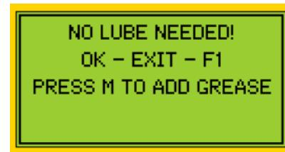
In case there is an **alarm assigned, and triggered**, you are informed that Lubrication Replenishment is needed. You have an option to continue in GUIDED MODE or FREE MODE. In case you want to ignore this recommendation and abort lubrication, you need to press M, assign the message and then exit.
