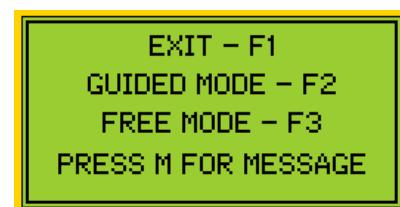
In case there is an **alarm assigned, but not triggered**, you are informed that Lubrication is not needed. You have an option to accept the recommendation done by alarm settings and press F1 to exit. In case you want to ignore this recommendation and continue, you need to press M, assign the message and then continue.
