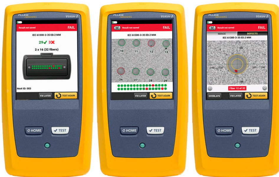
Seamlessly switch from a summary view (left) to an image (center), then use the gesture-based interface to zoom into a view of each individual fiber (right) and pan across the entire connector. Individual fibers are labeled so you know what you're looking at. Red defects are failures, green are acceptable per the selected standard.
