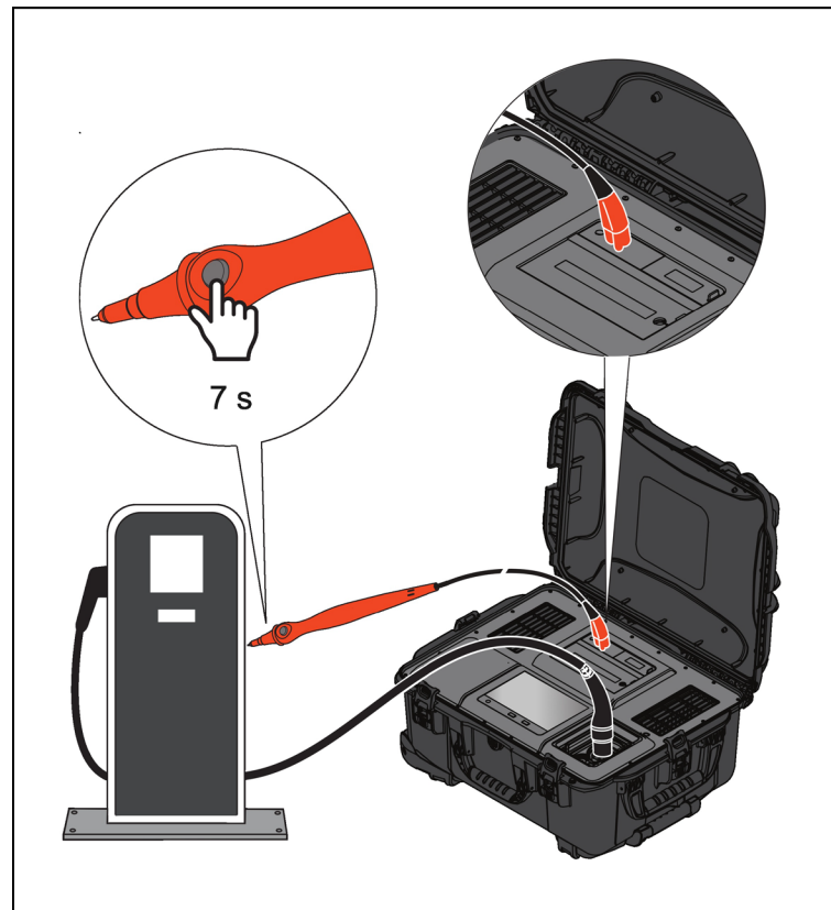
Figure 5. Performing Continuity Test
