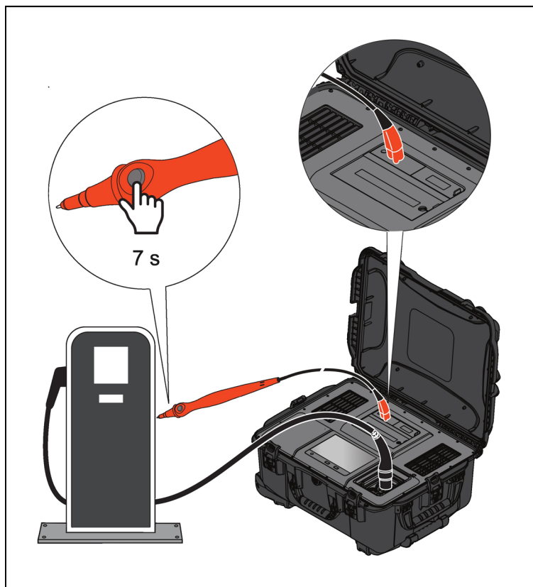
Figure 5. Performing Continuity Test
