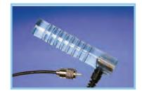
Electrode handle that attaches to the top of the meter. Can be used with the 830-series prods or the 831 short pin disc shaped prod. Useful for large or high density bales.
