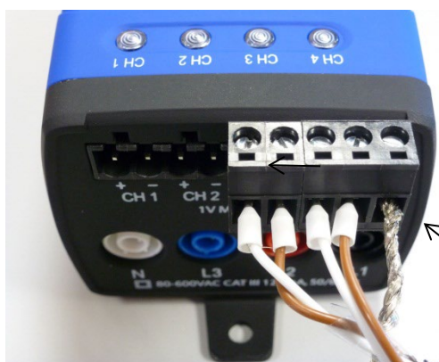
Connecting RōCoil CTs to an ELITEpro XC
