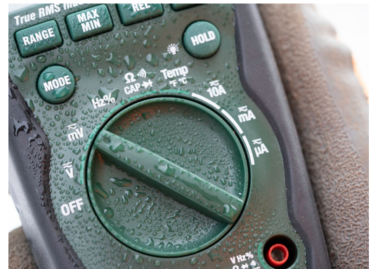
Double molded for rugged waterproof (IP67) protection
