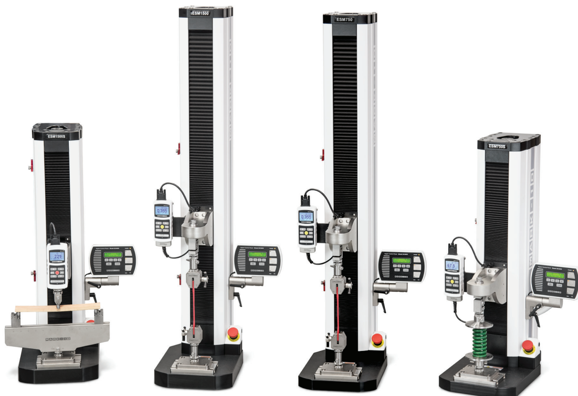
ESM1500S 1,500 lbf [6.7 kN] 14.2 in [360 mm] travel
