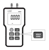
NOTE: Prior to use, the manometer must be zeroed. To do this, ensure the manometer is in a non-pressurized area and no hoses are attached.
