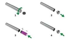
The EL-USB-1-RCG's battery is preinstalled. To charge the battery, connect to a USB port until the green LED shows. The rechargeable battery should only be replaced by an authorized supplier.
