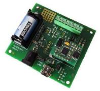
The EL-OEM-TEST is a board designed to assist in development of circuits using the EL-OEM-3 data logger.
