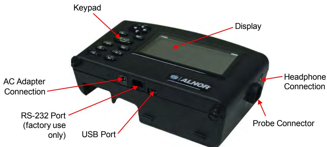
Figure 1: Features of the EBT730/EBT731 Micromanometer, Front View
