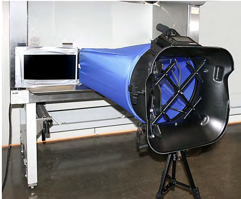
Figure 28: Adjust Height and Position of Telescopic Stand
