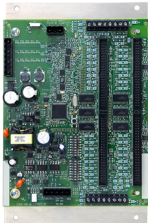
36/72-ch Bottom Feed Configuration Panel 1
