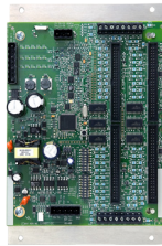
24/48-ch Bottom Feed Configuration Panel 1
