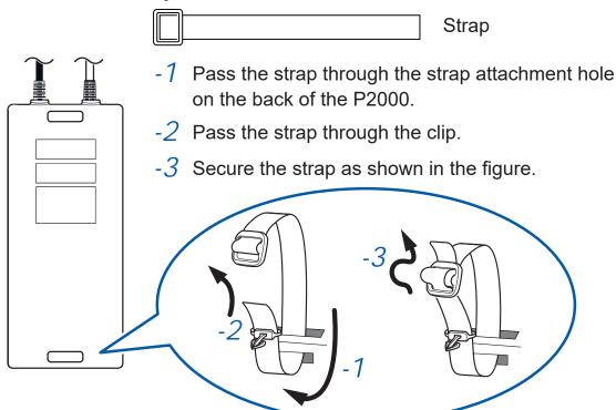
Attach the strap buckle to the strap holes (bottom) of the instrument and connect it to the clip that you attached to the P2000 with the strap.
