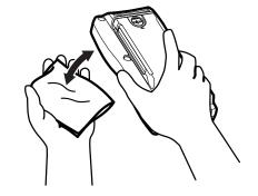
Securely hold the instrument with the measurement terminal facing down and gently tap the instrument against a soft cloth, etc. approximately 10 times until no water drops are coming out.
