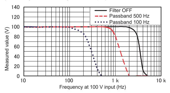
When measuring power supplies with a power frequency of 400 Hz, which is mainly used in ships and aircrafts
