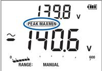
The maximum value of the peak value appears in the sub display and the minimum value of the peak value appears in the main display.
