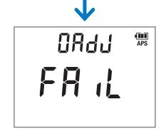
Screen displayed when zero adjustment fails
