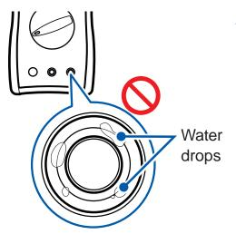
Check that there are no water drops inside the measurement terminals.
