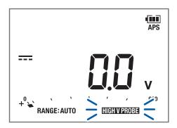
3 Connect the P2010 DC High Voltage Probe to the measurement terminals of the instrument.
