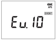
An event with a duration time of less than 200 ms may not be accurately measured, failing to detect the event.
