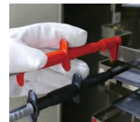
For clamping around the target busbar
