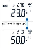
When the standard value is measured, press FILTER for at least 1 second.
