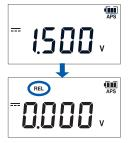
When the standard value is measured, press FILTER for at least 1 second.
