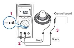
Example: Measuring the current of the burner flame ( $\mu A$ )
