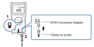
Set the clamp-on probe and the instrument to the same range.
