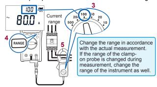
Measuring AC Current Using Clamp-on Probe (DT4253, DT4255, DT4256)
