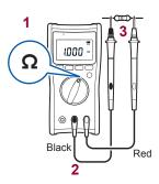
The open terminal voltage is approx. 1.8 V or less. The measurement current (DC) varies depending on the range. To avoid damage to the measurement object, check the specifications before use.
