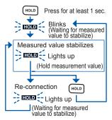
Press (HOLD) for at least 1 second. (HOLD blinks, the instrument is waiting for the measured value to stabilize.)
