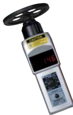
DT-207LR-S12 Contact Tachometer with Optional 12" Circle Wheel
