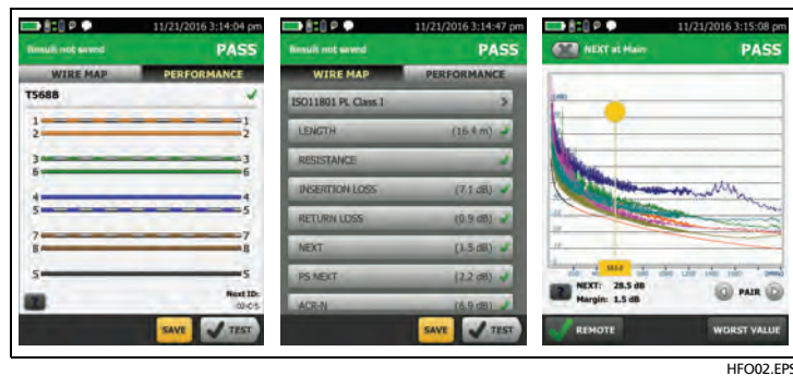
Figure 5. Examples of Twisted Pair Results Screens
