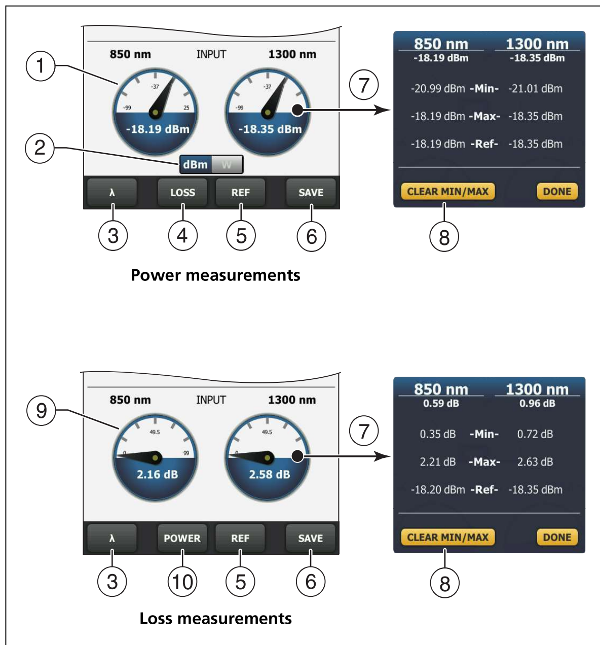
Figure 123. Power Meter Measurements and Controls
