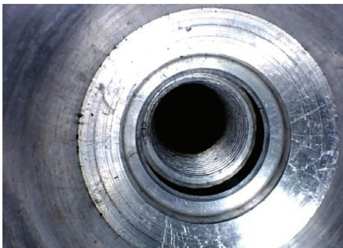
Photo above: Spark plug port inspection
