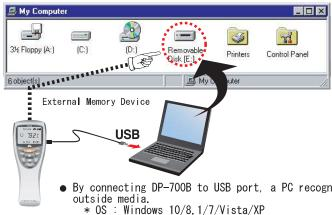
By connecting DP-700B to USB port, a PC recognizes DP-700B as
