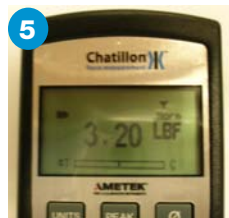
Observe Load Read the force result from the display. If you select the PEAK key after you complete your test, the DFX will display the maximum (Peak) load that was achieved during the test.
