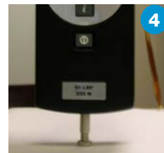
Apply Push Force Apply a pushing force to the sample under test. Observe the load bargraph (fills from the center towards the "C") and the Compressive Load Indicator (arrows). The main display will indicate the load being applied to the load sensor shaft using the fixture/adapter.
