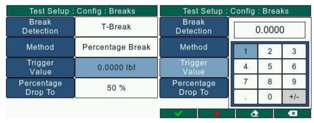
The user will have to exit the Configuration (ConfigurationScreen.html) screen and save changes for the trigger point setting to be applied.
