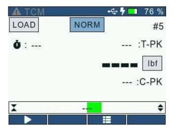
This function allows the user to "hide" the readings displayed on screen. The "hide" function is useful for blind study applications. This setting can be turned ON/OFF from the Test Setup: Display (TestSetupDisplay.html) screen.
