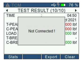
The results get exported only when the gauge to connected to a Serial Terminal like Termite. When not connected, the gauge will throw a "Not connected!" pop-up on the display.
