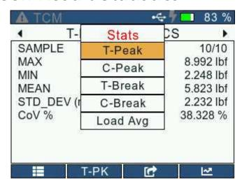
The F1 button can be pressed to get a list of available statistics and switch to the statistic to be viewed. The user can also switch between statistics using the Left/Right buttons.
