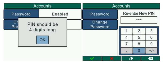
If the entered password is valid, the user will have to re-enter the new PIN to update the password. In case the passwords don't match, the gauge will throw an error message prompting the user.
