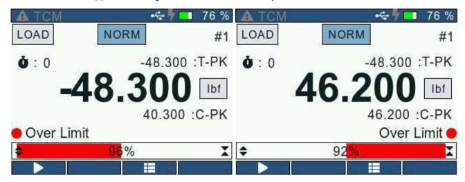
The Load Safety Limit can be configured from the Test Setup: Configure (TestSetupConfig.html) screen.
