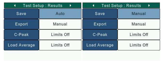
If the Save setting is Auto, the enabled results are stored automatically in the memory once a test is completed.
