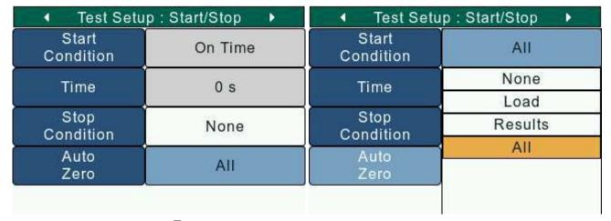
On the Test Setup: Start/Stop (TestSetupStartStop.html) screen, use the Navigation keys to set the cursor on the Lock Home setting. To change the Auto Zero setting, press the Select key to open a list with available options. The user will have to exit the Configuration (ConfigurationScreen.html) screen and save changes for the Auto Zero setting to change.
