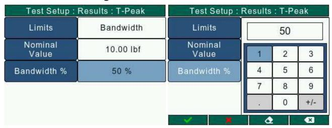
The Bandwidth Percentage determines the percentage of Nominal value that'll be added to and subtracted from the Nominal value in order to set the high and low limits respectively. The user must make sure that the entered value is such that the limits are lower than the maximum gauge capacity.
