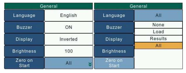
The DF3 Series allows the user to select one of the following readings as the Zero On Start option -
