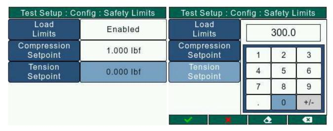
On the Test Setup: Config: Load Safety Limit (SafetyLimits.html) screen, use the Navigation key to set the cursor on the Tension Setpoint. To set the Tension Setpoint, press the Select key to open the numeric keypad (NumericKeypad.html). The user will have to exit the Configuration (ConfigurationScreen.html) screen and save changes for the Tension setpoint to set.
