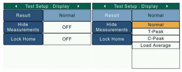
The available results depend on the Gauge Model and the tests that have been enabled in Test Setup: Config (TestSetupConfig.html).
