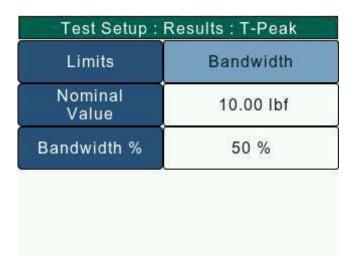
The Bandwidth method allows the user to set pass/fail limits with respect to a Nominal Value. Under this method, the user will set values for the Nominal value and Bandwidth percentage using the numeric keypad (NumericKeypad.html). Based on the inputs, the high and low limits are set as follows -
