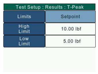
The Setpoint method allows the user to set high and low pass/fail limits. Under this method, the user will set values for the High and Low setpoints using the numeric keypad (NumericKeypad.html).
