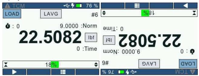
DF3 Series digital force gauges give the operator an option to invert the gauge display. This feature makes it easier for the user to analyze the readings when the gauge is held upside-down. When the display is inverted, the Navigation and Function key functionalities are swapped. The gauge display orientation can be changed from the General (GeneralScreen.html) screen.
