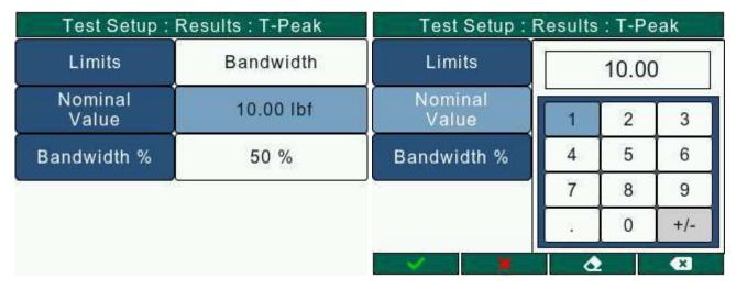
The Nominal Value determines the midpoint around which the bandwidth is calculated. The user must make sure that the entered value is such that the limits are lower than the maximum gauge capacity.
