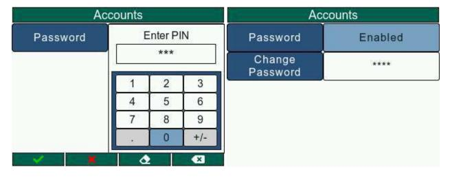
In case the entered password is incorrect, the gauge will throw an error message on screen and the setting will remain unchanged.
