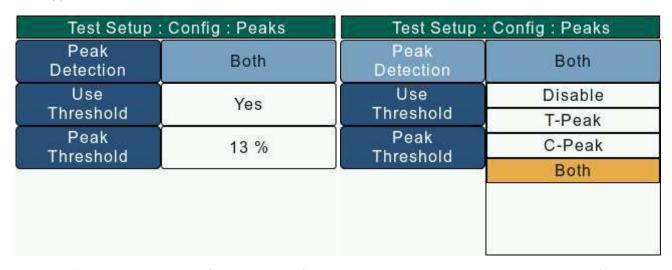
The user will have to exit the Configuration (ConfigurationScreen.html) screen and save changes for the Peak Detection settings to be applied.
