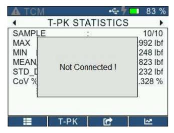
The Statistics get exported only when the gauge to connected to a Serial Terminal like Termite. When not connected, the gauge will throw a "Not connected!" pop-up on the display.
