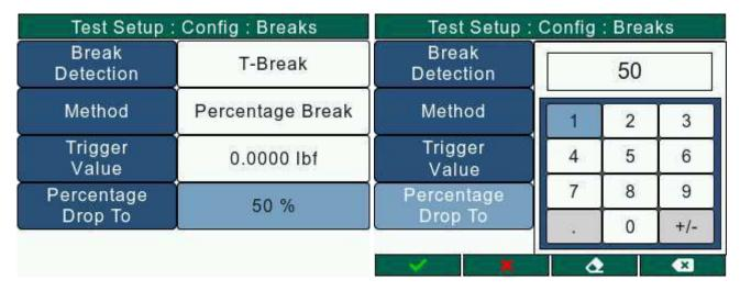
The user will have to exit the Configuration (ConfigurationScreen.html) screen and save changes for the percentage drop setting to be applied.
