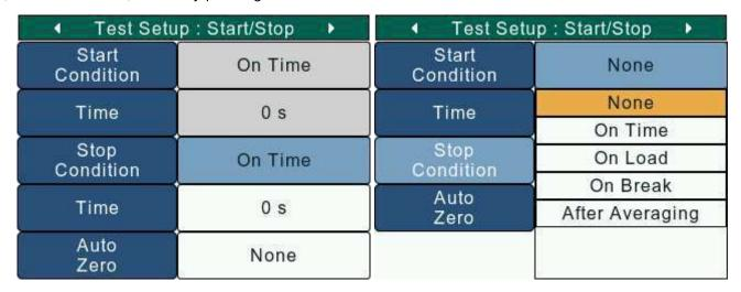
On the Test Setup: Start/Stop (TestSetupStartStop.html) screen, use the Navigation keys to set the cursor on the Stop condition setting. To change the Stop condition, press the Select key to open a list with available stop conditions. The available stop conditions will depend on the results that have been enabled in Test Setup: Configure (TestSetupConfig.html) screen.
