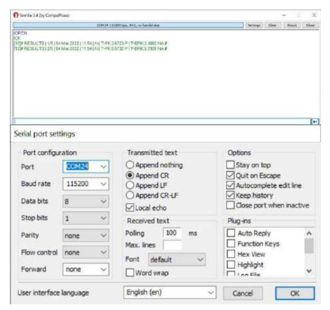
The gauge doesn't respond if there's an issue with communication. This could be because the gauge is being used by another application or the command sent is incorrect. Another reason could be a disparity in setting.
