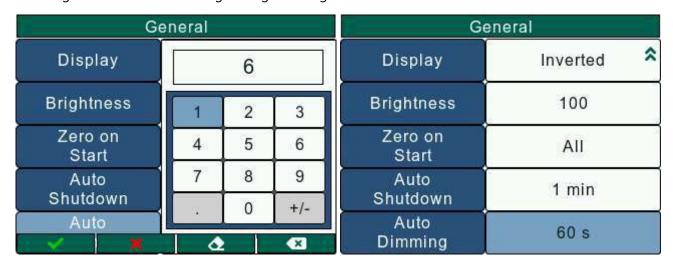
The user can set a value between 10 - 3600 seconds as the Auto Dimming timeout.
