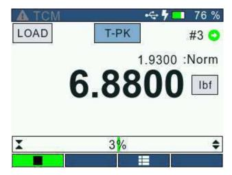
When the gauge is in Peak Tension mode (T-PK), the gauge will display the maximum tensile load that was measured by the loadcell sensor. In addition to that, the user will also be able to view the Peak Tension value as a sub-reading when the gauge is in Normal or Tension Break (T-Brk) (BreakDetection.html) Mode.
