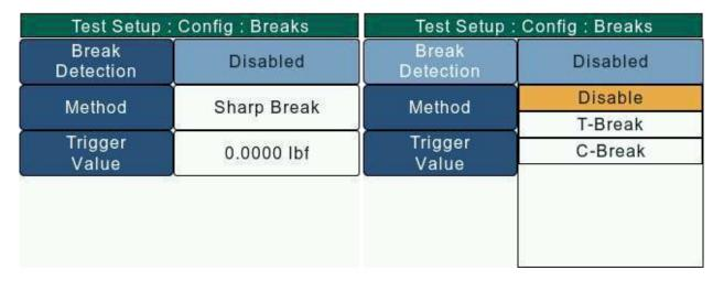
The user will have to exit the Configuration (ConfigurationScreen.html) screen and save changes for the break detection settings to be applied.
