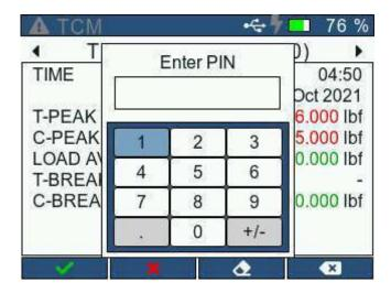
If the Password is enabled from the Accounts (./AccountsScreen), the user will have to enter the PIN before clearing the results.
