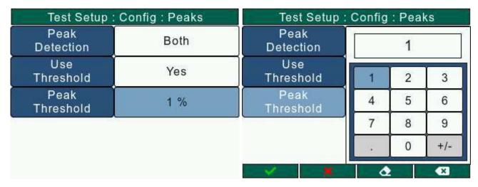
The user will have to exit the Configuration (ConfigurationScreen.html) screen and save changes for the Peak Threshold setting to be applied.
