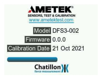
When the gauge is powered on, the Splash screen is displayed for approximately 5 seconds. This display shows AMETEK STC and Chatillon® logos along with Gauge Model, Firmware Version and the Last Calibration Date.
