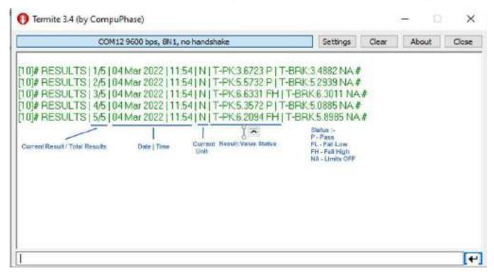
Before the exporting the results, the user must make sure that communication has been established with the serial terminal. To do this, the user must connect the gauge to the PC through USB and make sure no other application, such as ForceTest, DeviceAgent, is communicating with the gauge. Once this is confirmed, the user must send !OPEN command from the terminal and wait for the gauge to respond with !OK. If !OK is received, the user can go ahead and export results/statistics.
