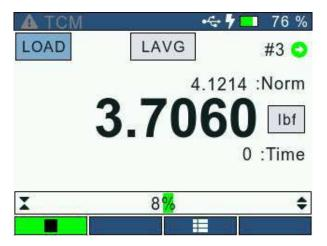
This load averaging test allows you to set a pre-load limit value or load threshold. The Preload value represents the "Start" and "End" point for your averaging function. The gauge will begin to collect and average the measured values once the "Preload Value" has been reached. The gauge will continue to average until the measured load drops below the Preload value. When the test is completed, the gauge will display the "Average Load".
