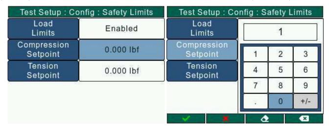
On the Test Setup: Config: Load Safety Limit (SafetyLimits.html) screen, use the Navigation key to set the cursor on the Compression Setpoint. To set the Compression Setpoint, press the Select key to open the numeric keypad (NumericKeypad.html). The user will have to exit the Configuration (ConfigurationScreen.html) screen and save changes for the Compression setpoint to set.
