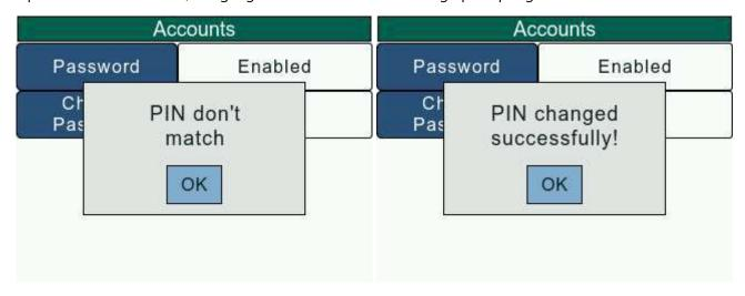
If the entered passwords are valid, the gauge will throw a 'PIN changed successfully' message and update the account password. The user will have to exit the Configuration (ConfigurationScreen.html) screen and save changes to change the password.
