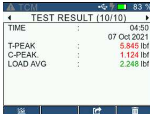
Saved results on the internal 32 GB SD card can be viewed and exported.
