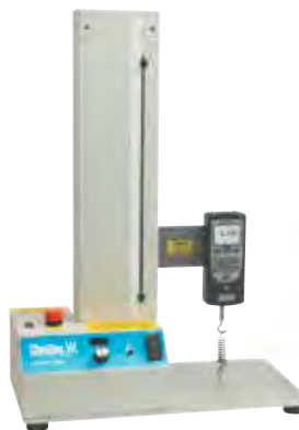
DFS II gauge mounted to LTCM100 tester
