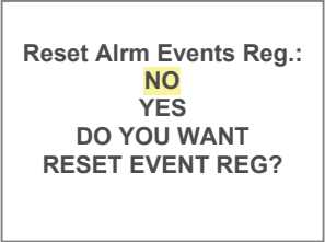
Figure 45: Resetting Alarm Events Register
