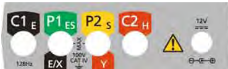
Test lead connections (at rear of instrument)
