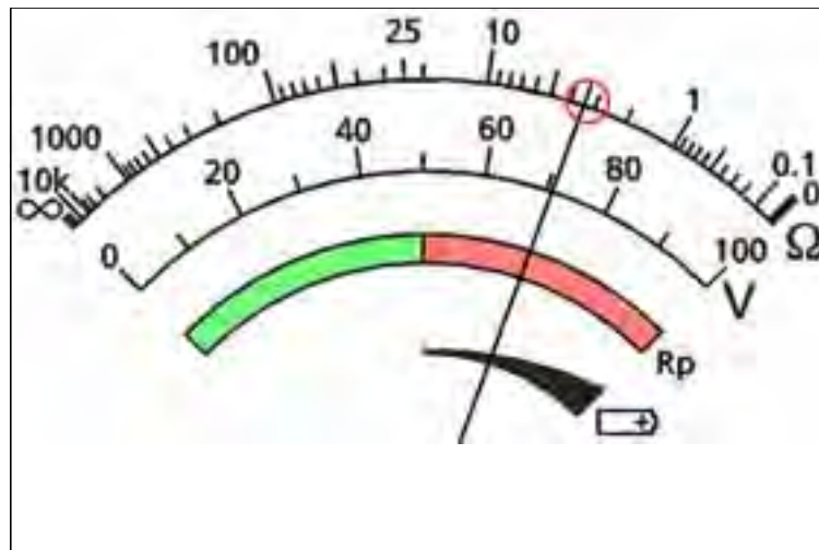
Figure 17: example two-terminal resistance reading
