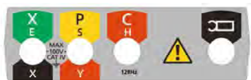
Test lead connections (at rear of instrument)
