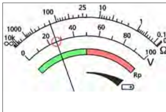
Figure 12: example ground noise voltage reading
