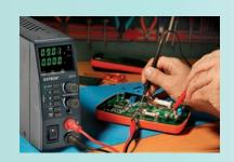
Extech's DCP36 power supply has 80W constant power topology and has autoranging Voltage and Current output. This compact and lightweight unit provides easy portability, and is ideal for tight workbenches with limited space. It features 4-Digit LED displays, 3-programmable presets, front/rear output terminals, and remote sensing for accurate applied voltage at load point.
