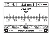
In the example, ruler mode shows the same situation as in figure **D**: Three steel bars equally apart. In rule mode, the clearance between the detected object centers can be determined.
