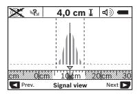
The object depth and the material types (as far as possible) are displayed. The maximum measuring depth is 6".
