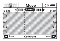
Position the detection tool against the wall and move it over the wall in the direction of travel (see "Operation Instructions", page 13). Measured results are indicated on display 16 after a minimum measuring distance of 4" (10 cm). To ensure correct measurement results, move the detection tool slowly and completely over the assumed object in the wall.
