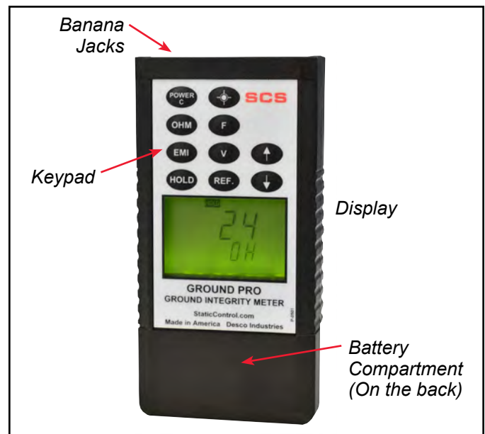
Figure 2. Ground Pro Meter features and components
