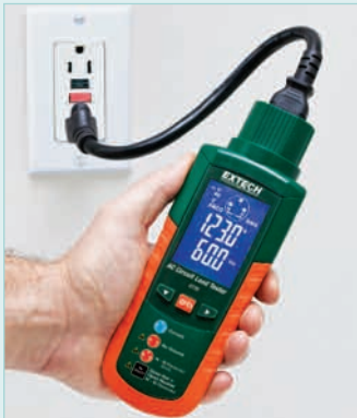
Tests 3-wire standard and GFCI receptacles
