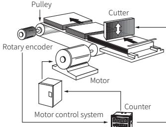
$$\text{Prescale value} = \frac{\pi \times \text{Diameter of pulley}}{\text{The number of pulses by 1 rotation of encoder}}$$
