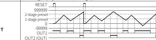
OUT1 output is off: counting display value  $\geq$  1-stage preset value.
