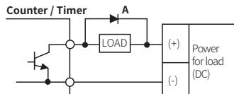
A: When using inductive load (relay etc.), surge absorber (diode, varistor etc.) must be connected between both sides of the load.
