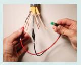
GREEN LED means wiring is properly identified.
